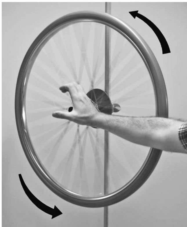
Figure 5.5. The bicycle wheel spins counterclockwise. The fingers of my right hand curl in the direction of the rotating wheel, while my thumb gives the direction of \vec{\omega} . (Photo by Jim Carico.)
