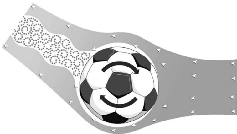
Figure 7.8. A sketch of a soccer ball spinning clockwise. The ball moves from left to right, meaning that the air flow is right to left. Note how the boundary layer separation is delayed on the bottom of the ball.
