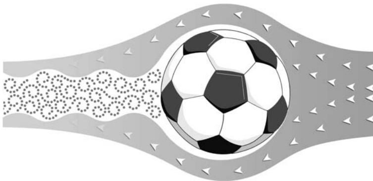
Figure 7.6. The soccer ball in the sketch here moves faster than the one in Figure 7.4. Note the delay in the boundary layer separation. The air flow is turbulent.
