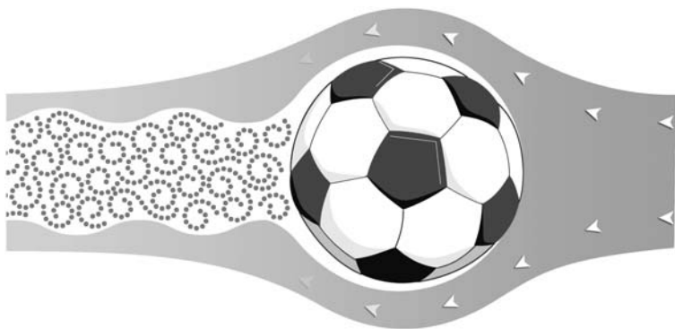
Figure 7.4. A sketch of a soccer ball moving through the air, but viewed in the ball's reference frame. The ball moves from left to right, meaning that the air moves from right to left from the ball's point of view. Note the many eddies behind the ball. The air flow is "laminar."
